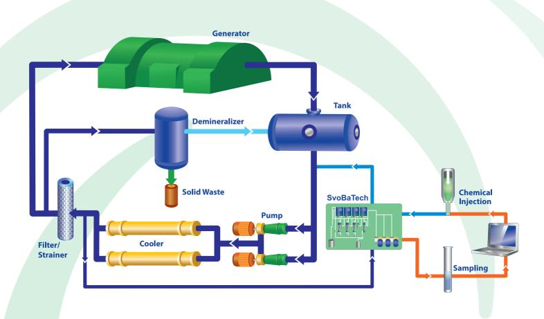
With the longest experience in the industry, we are specialized in the chemical cleaning of water-cooled generator coils and the stator cooling water system. Our method is based on the use of chelants (e.g. EDTA) with innovative developments built on 40 years of industry knowhow. Chelant cleaning removes copper oxides without attacking the system materials. The process employs dedicated monitoring of the process parameters,
